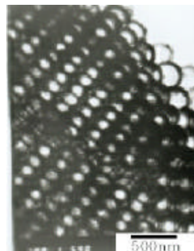
Figure 3 TEM image of the macroporous ZnS, taken with Hitachi H-800 microscope operated at 200kv
